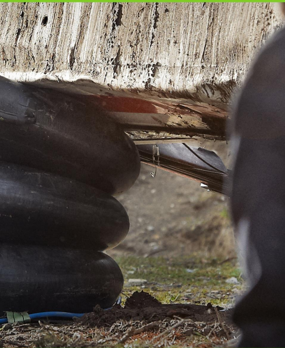
The ProFix Max provides 10 ton lifting capacity by integration of the ram.
